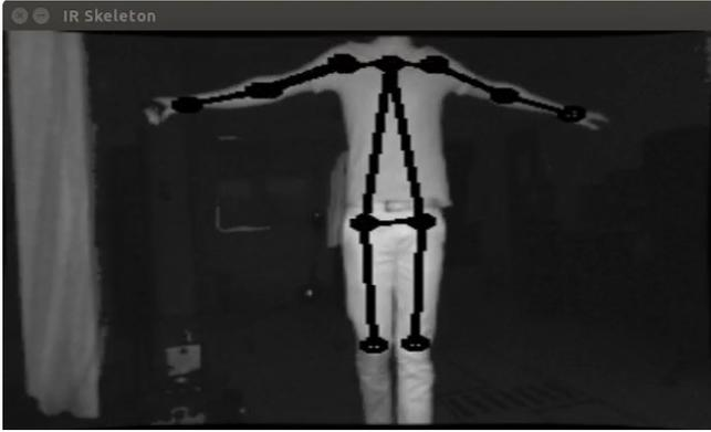
Fig. 9: Exemplification of skeleton detection on infrared images
