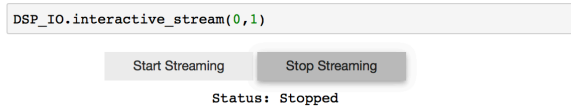
Fig. 5: Setting up an interactive stream for the simple y = x loop through, using a run time of 0, which implies run forever.
