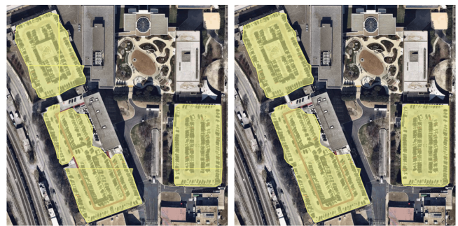
Fig. 12: Left: Polygons crossing tile boundaries, and other adjacent polygons, are combined. Right: Combined polygons.
