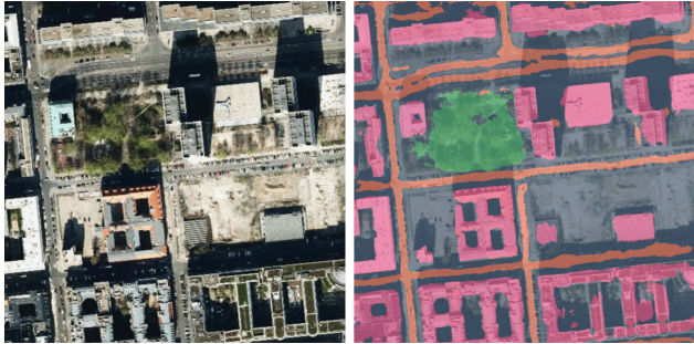
Fig. 7: Left: Original satellite image. Right: Semantic segmentation of roads, buildings and vegetation.
