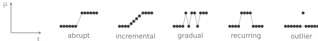
Fig. 2: Drift patterns depicted as the change of mean data values over time. Note that an outlier is not a change but noise in the data. This figure is based on [GZB + 14].
