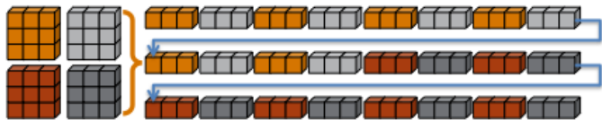
Fig. 7: Flattening a 2D distributed array. The block owned by a process becomes discontinuous when representing the 2D array in 1 dimension.
