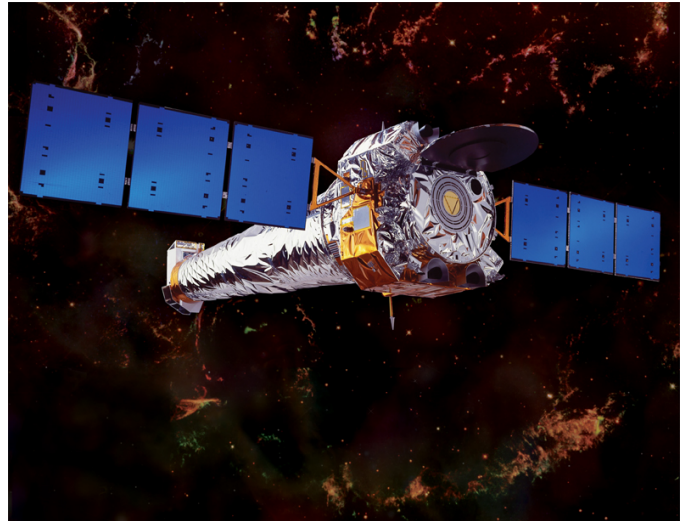
Fig. 1: Artist's rendering of the Chandra X-ray satellite. The silverized teflon which wraps the spacecraft has degraded so it is now far less reflective than shown.
