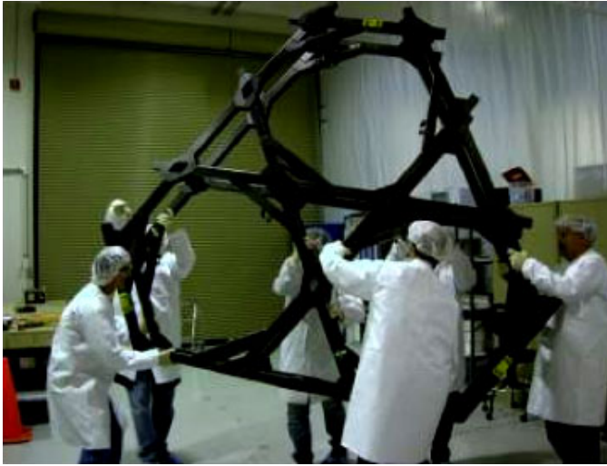
Fig. 2: Engineers move the Backplane Stability Test Article (BSTA) into position for the thermal vacuum test. This test piece represents a section of the backplane that will support only 3 of the 18 mirror segments of the primary mirror for JWST.
