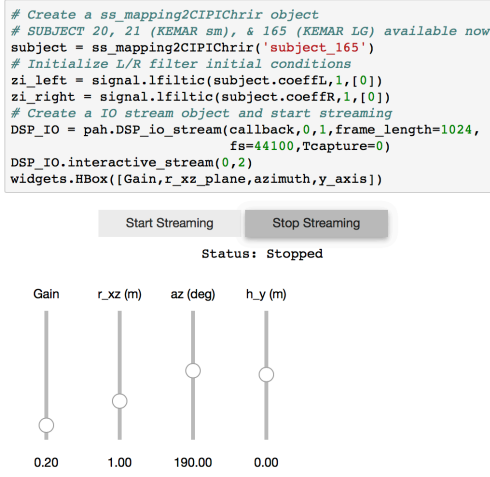
Fig. 7: Jupyter notebook for static positioning of the audio test source.
