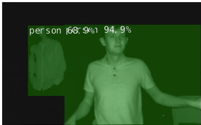
Fig. 8: Exemplification of people detection on infrared images based on detection
