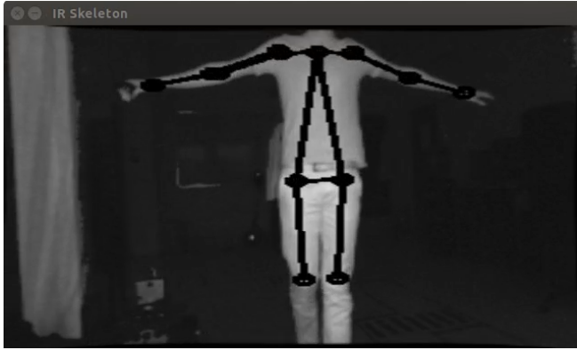
Fig. 9: Exemplification of skeleton detection on infrared images
