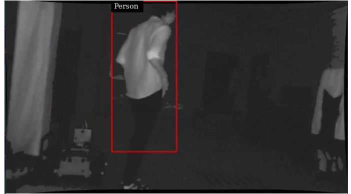
Fig. 10: People detection algorithm running with the Deepstream SDK on the Jetson Xavier NX board
