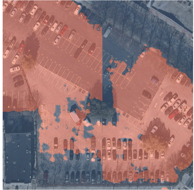
Fig. 11: An example of border artifacts and holes in raw segmentation masks produced by our U-Net model.
