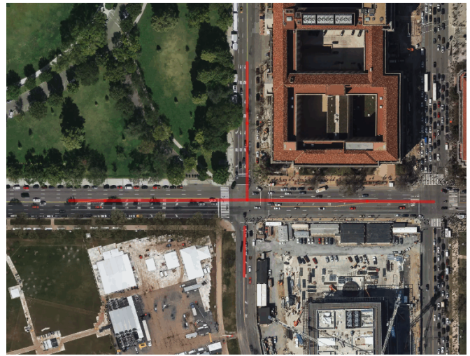
Fig. 3: A custom layer created by clipping the locations of roads with turn lane markings to Mapbox Satellite. Streets with turn lane markings are rendered in red.
