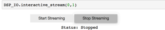
Fig. 5: Setting up an interactive stream for the simple y = x loop through, using a run time of 0, which implies run forever.
