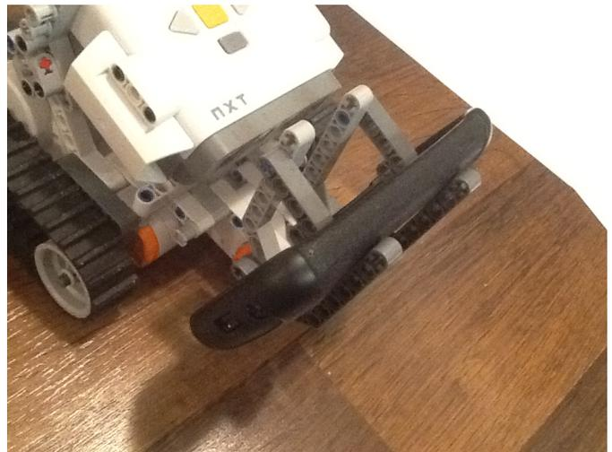
Fig. 2: A close up look at the holder mechanism for the Android phone.
